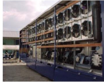
2. Pre-cooling in the field by mobile hydro coolers, decreasing temperatures to 2°C in under 10 minutes
