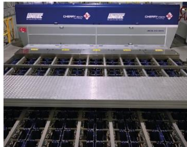
3. State of the art electronic sorting and sizing with in-line hydro cooler
