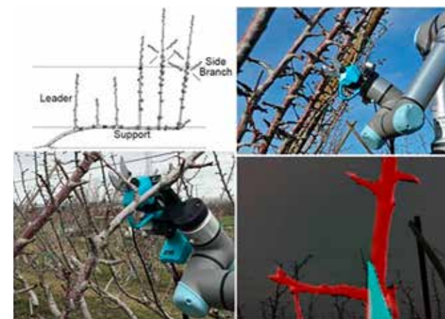
Fig. 1. (Top left) A diagram of a UFO cherry tree structure, including the side branches to be pruned from the vertical leaders. (Top right and bottom left) Our pruning robot uses a manipulator mounted on a mobile base with an eye-in-hand RGB-D sensor and electric bypass shears. Bottom right) Segmented image taken during the approach to the pruning point.
