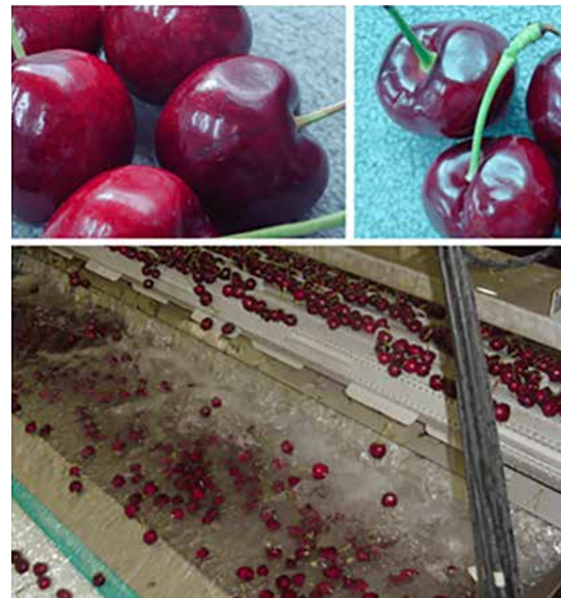
Image 2. Damage caused by insufficient amount of water used in transits during processing.
