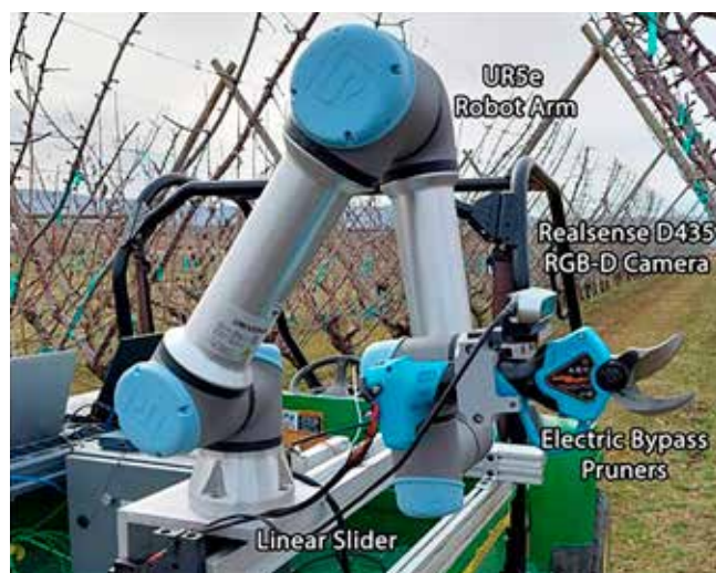
Fig. 2. Our pruning setup, consisting of a Universal Robots UR5e robot mounted on a linear axis. The end effector consists of a set of electric bypass pruners along with a RealSense D435 RGBD camera.
