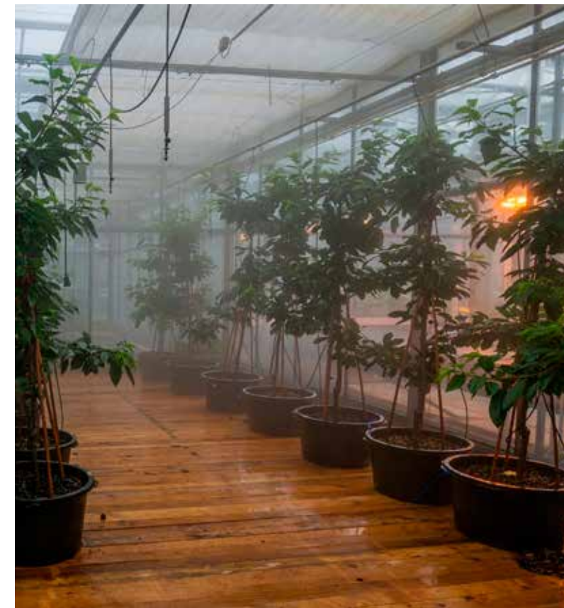
Image 2: Fog chamber to simulate rain.
